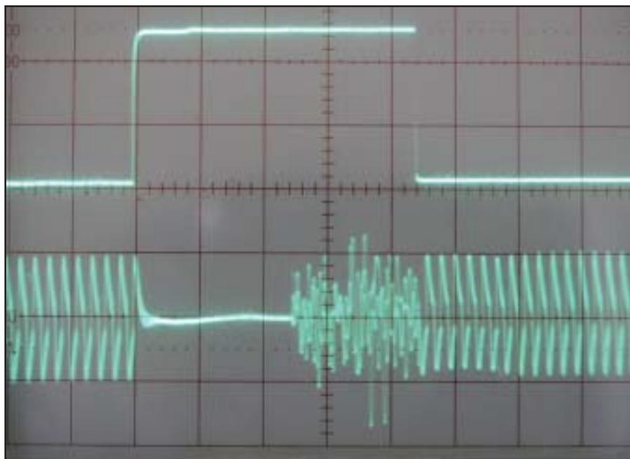
Figure 3 — Here the low frequency sine wave has been eliminated. No transient in the audio output, just receiver noise.
